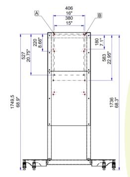
A: The Mobile Stand Mix® has 2 mounting positions for the BalanceBox® 400 or the Universal VESA Bracket:
